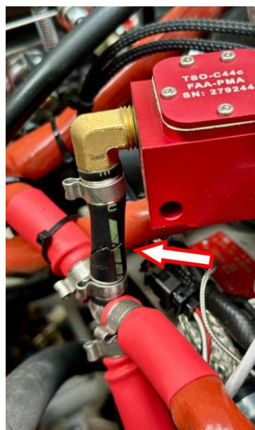
Cracks have been found on various fuel hoses installed on some SHARK aircraft.
